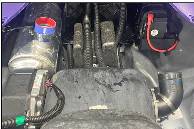
Insert straight end of supplied exhaust tube into exhaust outlet until you feel it lock in place.
