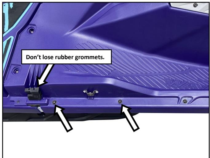
While raising rearmost edges of center deck section, carefully remove rear deck section completely and set aside.
