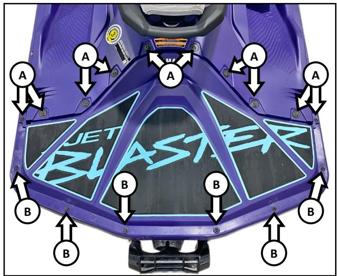
Remove bolts (6 - B) securing rear deck section to hull.
