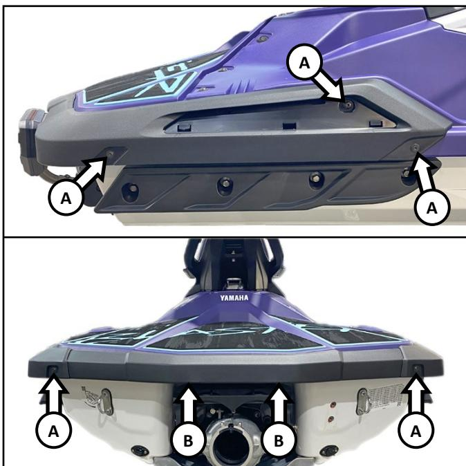
Remove rear bumper (2 nuts - B) and set aside. **TIP:** Disconnect reverse cable from reverse bucket (left side of jet pump) and lower reverse bucket by hand.
