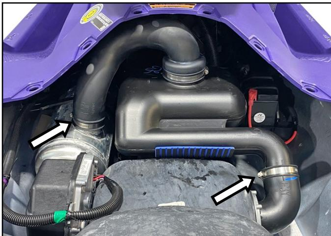
Remove exhaust baffle assembly and discard.
